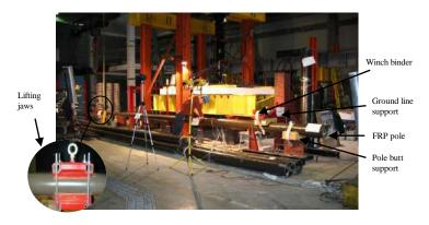
Figure 1 Full-scale test setup.
