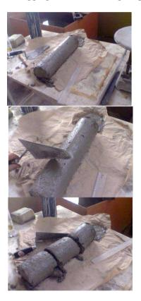
Figure 4 Steps of Static Segregation Index test:
