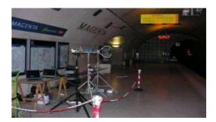
To this end, three experiments have been carried out, in order to find the influence of two different parameters, namely ventilation and trains on the pollutant concentrations. These experiments took place by night when public access is forbidden in order that these three parameters could be individually investigated.
