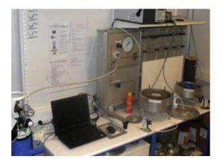
Picture 1 Gas permeameter CEMBUREAU, (GeM Laboratory – France)
