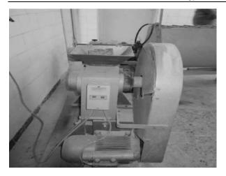
Figure 3 Jaw crusher apparatus and the machine in operation
