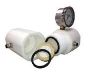
Figure 1 Two-chambers diffusion cell, sample and rubber rings.
