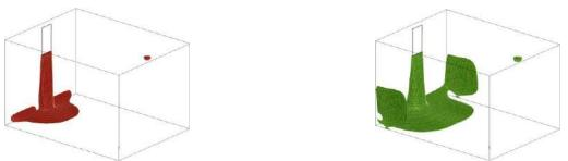
Fig. 4. Contour plots of iso-velocity with:  $0.25 \text{ m.s}^{-1}$  (*left*) and  $0.15 \text{ m.s}^{-1}$  (*right*)
