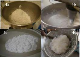
Figure 4 Binders: 4a) plaster powder; 4b) plaster binder; 4c) starch powder; 4d) starch binder
