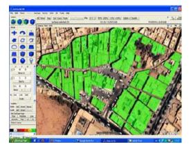
Figure 3 Tracing the complex urban morphology using AC3D
