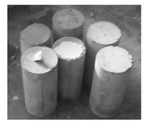
Figure 2 Test specimen as concrete waste
