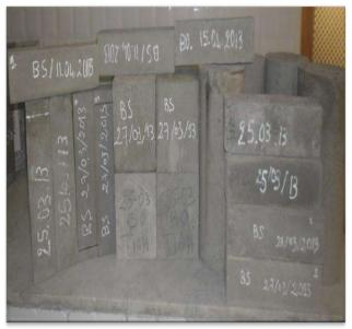
Figure 2 Concrete specimens
