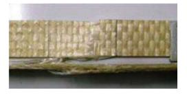
Figure 5 Breaking mode by tensile test of laminate
