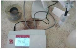
Figure 5 Calibration of conductimeter with a KCl solution.
