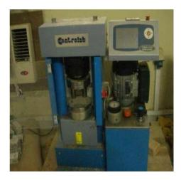
Figure 2 Machine testing compression-flexure 50 kN Class 1.
