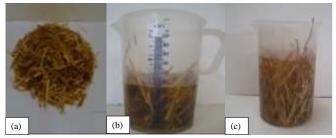
Figure 1 Straw fibers treatment: (a) crushed straw, (b) linseed oil immersion, (c) boiled water immersion.
