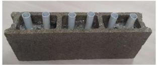
Figure 2. Photography of the block filled with PCM and ventilated tubes
